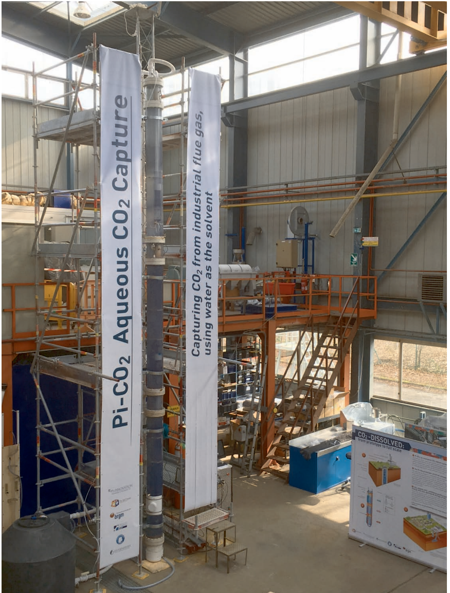
Figure 4 – The ‘Pi-CO2’ water-based CO2 capture technology prototype undergoing testing at BRGM’s experimental laboratory (© BRGM – Rowena Stead)
