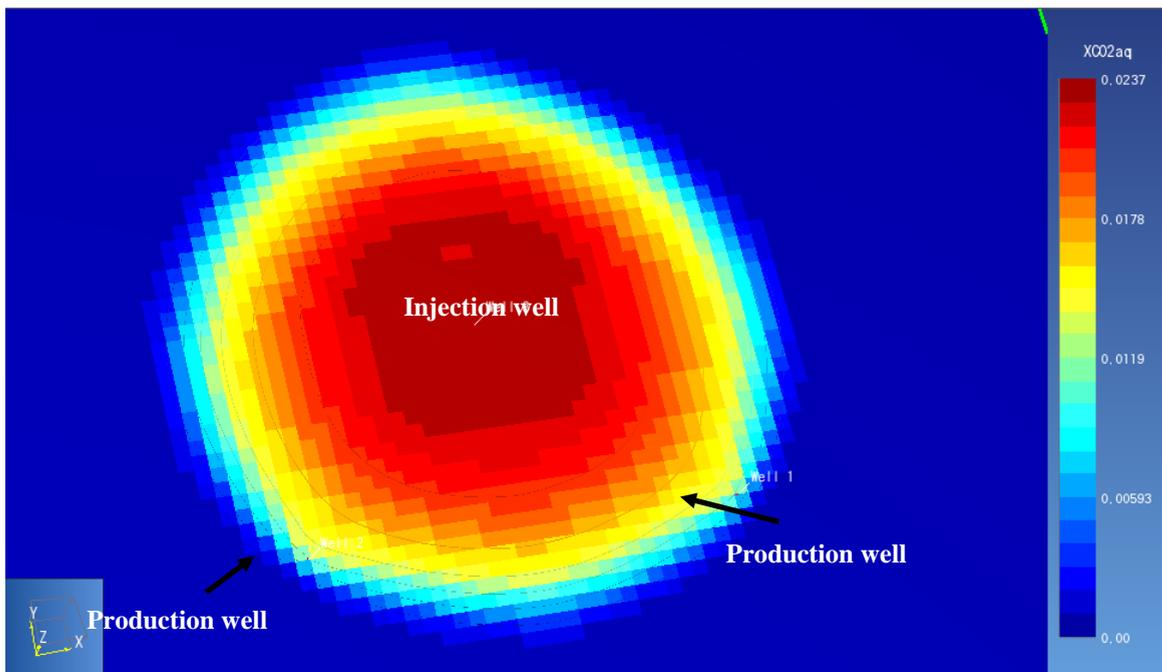
Fig.3. Simulated CO<sub>2</sub> mass fraction in the brine after 30 years of CO<sub>2</sub> co-injection operations.
