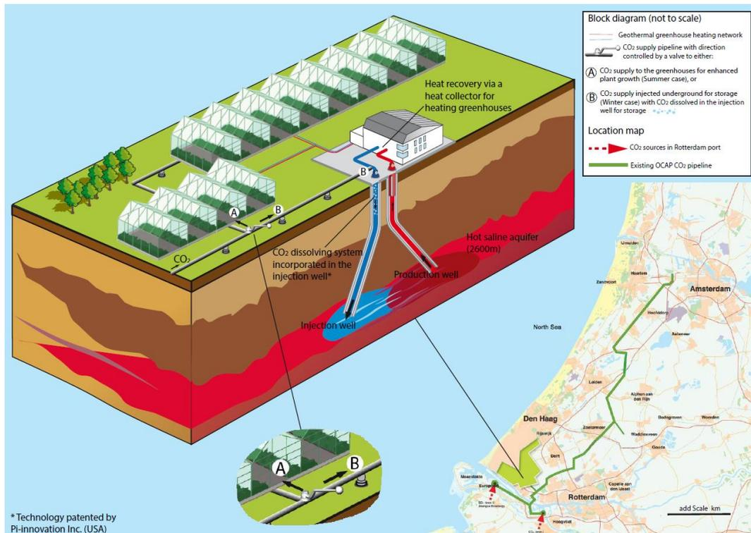
Fig.2. Location of the proposed pilot site in the Westland area in The Netherlands; inset: Switching valve between the CO<sub>2</sub> feeding circuit and injection circuit.
