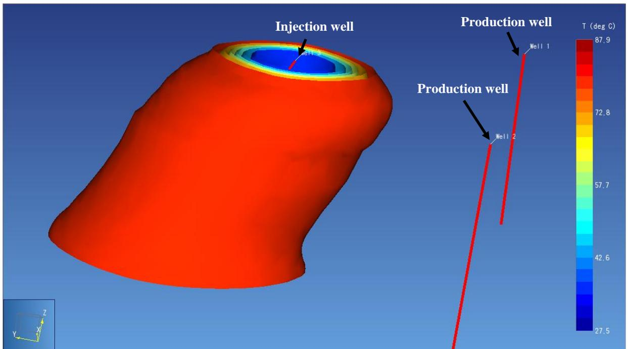
Fig.4. Temperature of the brine after 30 years of CO<sub>2</sub> co-injection operations.
