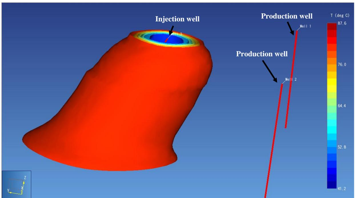
Fig.5. Temperature of the brine after 30 years of conventional operations without CO<sub>2</sub> co-injection.
