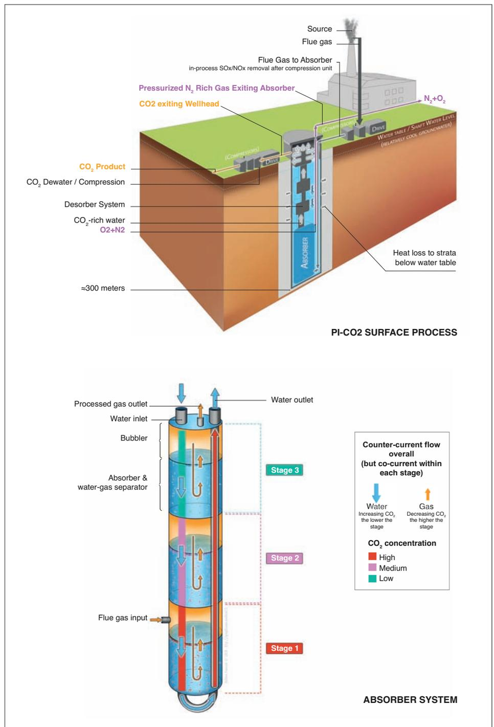
Figure 2: Pi-CO<sub>2</sub> Surface and Subsurface System Schematic (© BRGM - Hélène Fournié 2018 <http://graphisme-medical.fr>)
