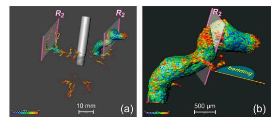
**Figure 15.** 3D model of the mean curvature distribution, H, for (a) the entire dissolution pattern and (b) the principal wormhole. Maximally and minimally curved areas are shown in red and in blue, respectively.
