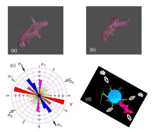
**Figure 12.** Skeleton model from CT 3D visualization of the principal wormhole represented as the (a) bottom and (b) vertical view of experiment #7. (c) Rose-diagram depicting the preferential directions of the growing principal wormhole, (d) which is shown in pink in the top view of the 3D model.
