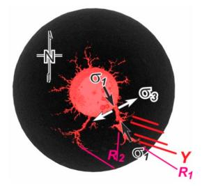
**Figure 10.** Results of structural interpretation of the dissolution network/wormhole morphology for experiment #6 (24 h CO<sub>2</sub>-rich solution injection into the sample).
