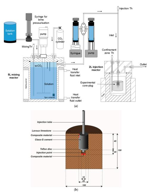
**Figure 1.** (a) Experimental device (MIRAGES-2) used to inject the CO<sub>2</sub>-rich solution in the core-plug under controlled conditions of pressure, temperature, and flow rate; (b) schematic view of the core-plug and the injection well. Dimensions are provided in millimetres.
