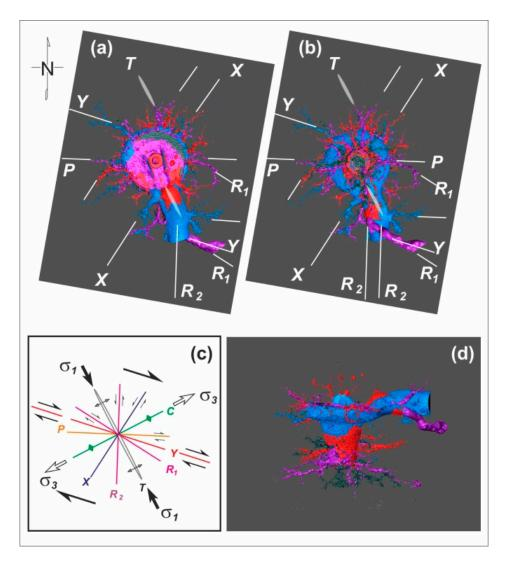
**Figure 8.** Azimuthally referenced structural control of dissolution arrays and principal wormhole morphology derived from the results of a spatial comparison of the experimental results: #1 (shown in grey), #2 (shown in purple), #3 (shown in red), #4 (shown in blue) in the framework of depicted orientations of fractures (**c**) appeared to be pronounced in the original sample of Lavoux limestones: (**a**) top view; (**b**) bottom vertically mirrored view; and (**d**) side 3D view.
