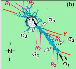
**Figure 9.** Results of structural interpretation of dissolution network/wormhole morphology for experiment #9 (12 h of  $CO_2$ -rich solution injection into sample): (a) 3D model and (b) top view of the 3D model after CT inspection, horizontally cut at the level of the orange dashed line within inset (a).
