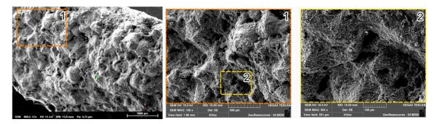
**Figure 14.** Multiscale Scanned Electronic Microscope (SEM) details of conical slickolites within the wall of the R<sub>2</sub> shear within the studied sample (experiment #7).
